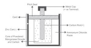
There is a brass cap on the carbon rod. zinc can be insulated by a piece of cardboard. A thick layer of pitch makes the cell insulated at th top.
