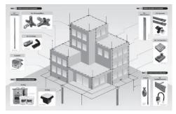
Whenever a loud with an electric charge passes over the building, an equal and opposite charge is built on the pointed end of the lightning conductor at the top of the building. This charge cannot be held up by the metal and all of it goes safely to the earth through the metal rod. Thus, the cloud also loses its charge. In this way, when lightning strikes the building, it flows to the earth through the metal rod of the conductor and prevents the building from getting damaged.
